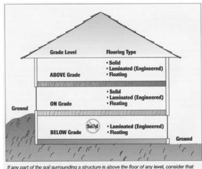
If any part of the soil surrounding a structure is above the floor of any level, consider that level below-grade. This includes walk-out basements. In addition, the surrounding soil should be sloped away from the structure with at least 6 inches of fall over the first 10 fee
