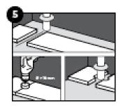
In rows where there is a pipe, make sure the pipe falls exactly in line with the short side of two planks. Take a drill bit with the same diameter as the pipe plus 16mm (0,63inch). Click the planks together on the short side and drill a hole centered on the joint between the two planks. Now you can install the planks.
