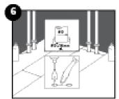
In case of a double pipe, drill a hole at each of the marked points that is equivalent to the diameter of the pipes plus 16mm. If located on the long side of the plank, make a 45 degree cut from each hole to the edge of the plank.
