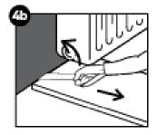
When sawing the panels make sure that the expansion gap under the door is 8mm. If you cannot lift the panel (e.g. under radiators), use the tapping block or pull-bar to tap the planks together.
