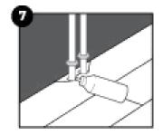
Then, using an appropriate PVC glue along the cut edges of the piece you cut out, glue the piece in place. Be sure no glue comes between the cut out piece and the subfloor. For a perfect finish around pipes, use pipe covers.
