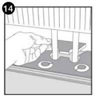
Fig 13 and 14. Installation at radiators. Drill the holes 2 x spacer thickness larger, than the diameter of the pipes.
