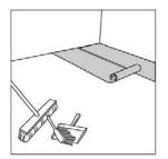
After thoroughly cleaning the subfloor, you should install a foam underlay (unless your product has a pre-attached pad). Run the foam underlay in the same direction as the flooring planks. The underlay should be butted side-by-side with no overlap. Tape seams together. If you are installing over a concrete suboor, a 6-mil poly (plastic sheeting) is to be installed under the foam underlay. (Many foam underlays already have this plastic sheeting pre-attached).
