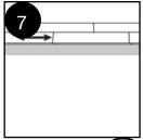
Staggered joint distance i.e. minimum distance between short ends of planks in parallel rows should NOT be less than the given width of the plank.
