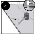
Afterwards use a rubber mallet along the tongue side of the short end to engage the planks. Please be careful not to damage the profile or edges during engaging the planks. Test each end joint to make sure it is completely engaged.
