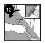
Cut off the vertical locking part of the strip with a chisel, put applicable glue on the strip and push the planks horizontally together. If necessary place some spacers between last board and the wall during the hardening.
