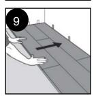
After 2-3 rows. Adjust the distance to the front wall by placing 10mm spacers.
