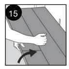
Separate the whole row by carefully lifting up and release the whole row.
