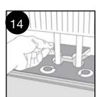
Installation at radiators. Drill the holes 2 x spacer thickness larger, than the diameter of the pipes.
