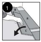
First row. Place a panel (A) as support for long side alignment of panel (B) and (C) while you install panel (B) and panel (C). Place a 10mm spacer between panel (B) and the wall. After that the complete first row is installed, remove panel (A) and slide the first row up against the wall with 10mm spacers placed between the panels and the wall.
