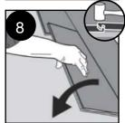
Second plank second row. Place the panel gently and close to the short end of the previous panel and fold it down in a single action movement reinforced with a rubber mallet as in step 4.
