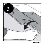
Fold it down with a single action movement. During the fold down, make sure the panels are close to each other.
