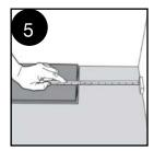
At the end of the first row, put a spacer to the wall and measure the length of the last plank to fit. Cut the extra material and complete the row.
