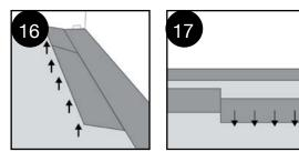
Disassemble the panels by lifting the short ends upward and then slide. Do never fold up a panel, as this damage the profile.
