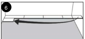
After 2-3 rows. Adjust the distance to the front wall by placing 10mm spacers.
