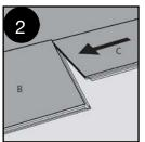
Second plank, first row. Place this plank (C) gently close to the short end of the first one (B).
