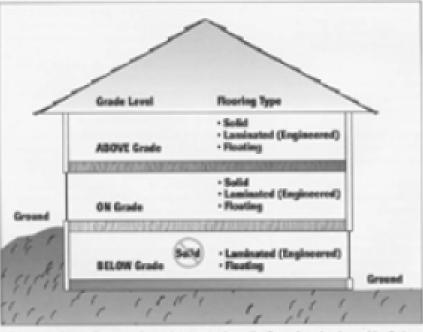
If any part of the soil sumounding a structure is above the floor of any level, consider that level below-grade. This includes walk-out basements, in addition, the surrounding soil should be stoped away from the structure with at least 6 inches of fail over the first 10 feet.
