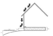
NOTE: Proper drainage away from the structure is absolutely critical to ensure weather-tight conditions and crucial to proper hardwood flooring performance. If structure is near a hill, the lot should be graded with a swale to move moisture off the lot and prevent it from coming in contact with the foundation.
