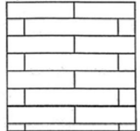
**E. Mechanically fastened strip and plank.**
