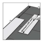
**Step 3** Cutting and fitting of final plank in first row
