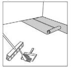
by-side with no overlap. Tape seams together. If you are installing over a concrete suboor, a 6-mil poly (plastic sheeting) is recommended to be installed under the foam underlay. (Many foam underlays already have this plastic sheeting pre-attached).
