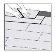
**Step 6** Measure and cut final row of planks allowing for 5 mm expansion gap
