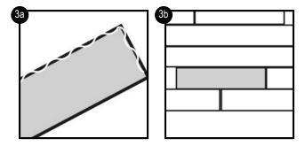
Apply glue on the cut groove side to adhere to the adjacent planks.
